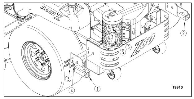
Bagger Brackets and Muffler Deflector Assembly Figure 1-8
